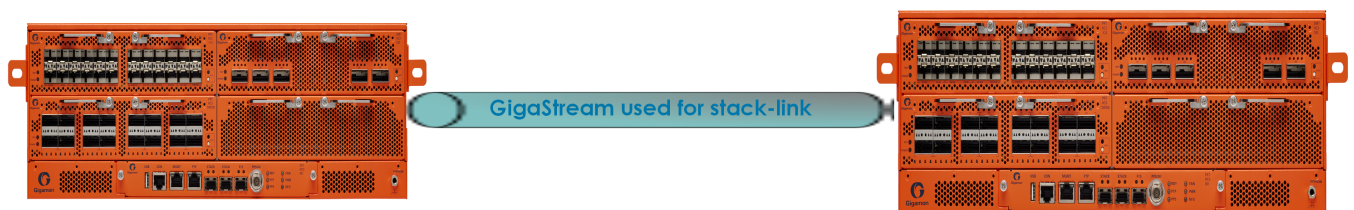
Figure 4 Daisy-Chain Configuration using GigaStream for Stack-link
