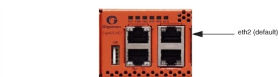
Figure 107 Stack Port Location on GigaVUE-HC1 Front
